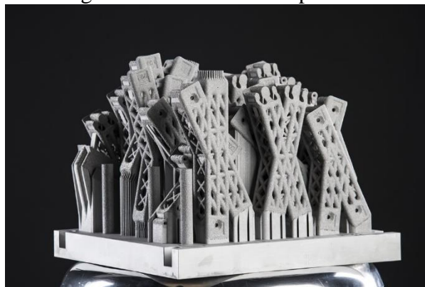
Fig. 11. Final printed piece– part of a bionic aircraft partition by Airbus [27]
