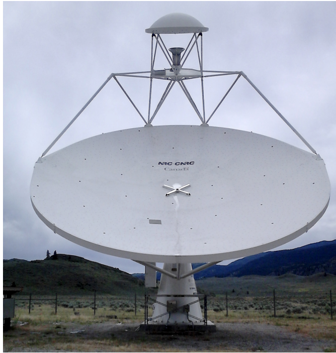
FIG. 27. Prototype SKA fiberglass dish, located in Canada at the Dominion Radio Astrophysical Observatory
