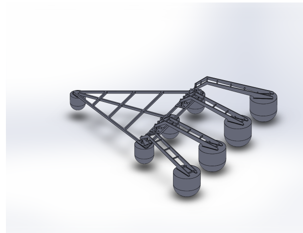
Fig. 1. 3-D view of the 8 floats 1-3-4 M4 configuration.
