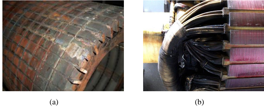
Fig 2.5: Rotor failures in induction machines: a) squirrel cage rotor, b) wound rotor [74]
