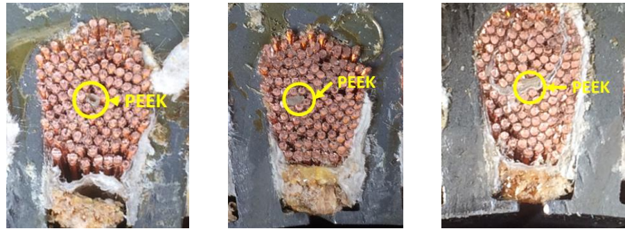
Fig 3.37: PEEK capillaries position in the slot centre
