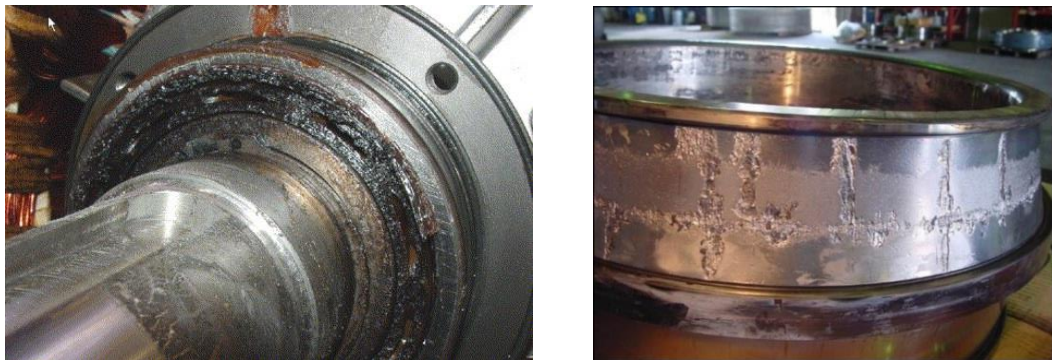
Fig 2.6: Bearing failures damage in rotating electric machines [77, 78]
