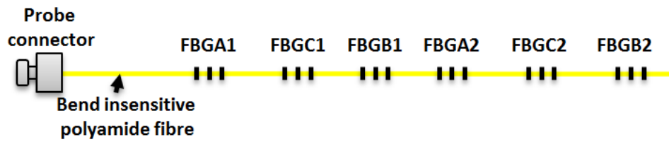
(a) FBG array design for radial distributed thermal sensing in TEFC-IM
