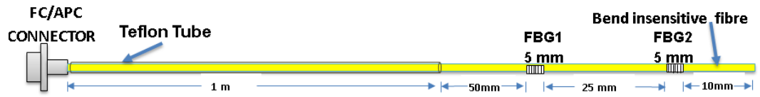
(b) FBG array design for rotor instrumentation
