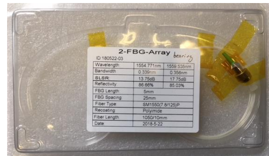
(b) Array FBG with 2 FBG heads
