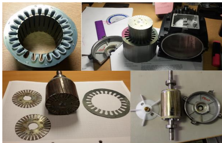
Fig 3.1: Disassembled motor and dimensions measurement for Motor-CAD model inputs
