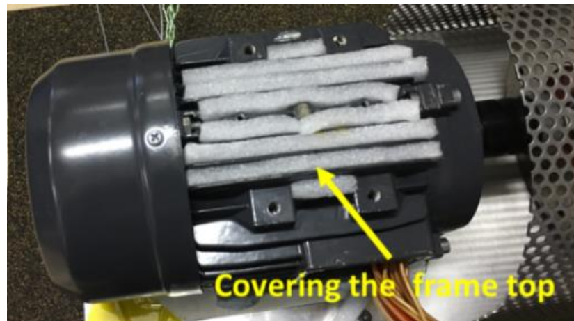
Fig. 8: Test motor with coated upper frame
