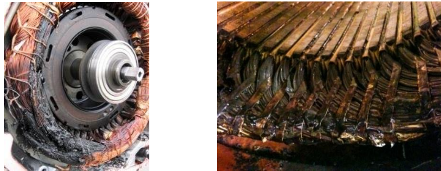
Fig 2.3: Stator winding failures in a slot and an end-winding section [67]
