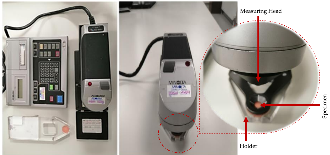
Figure 3.7. Pictures illustrating Minolta Chroma Meter instrument. Measurement of colour change of specimen performed in the holder of Chroma Meter (inset).
