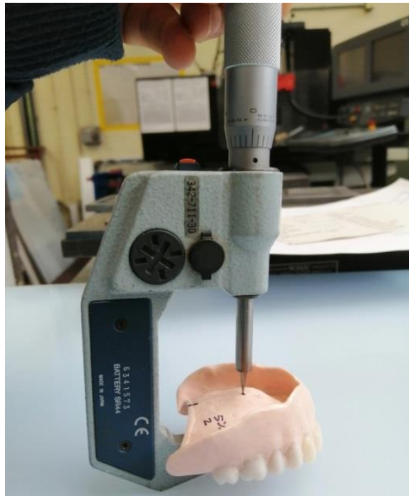
Figure 3.20. Photograph showing the denture thickness measurement using a micrometer at the point of loading during bending test
