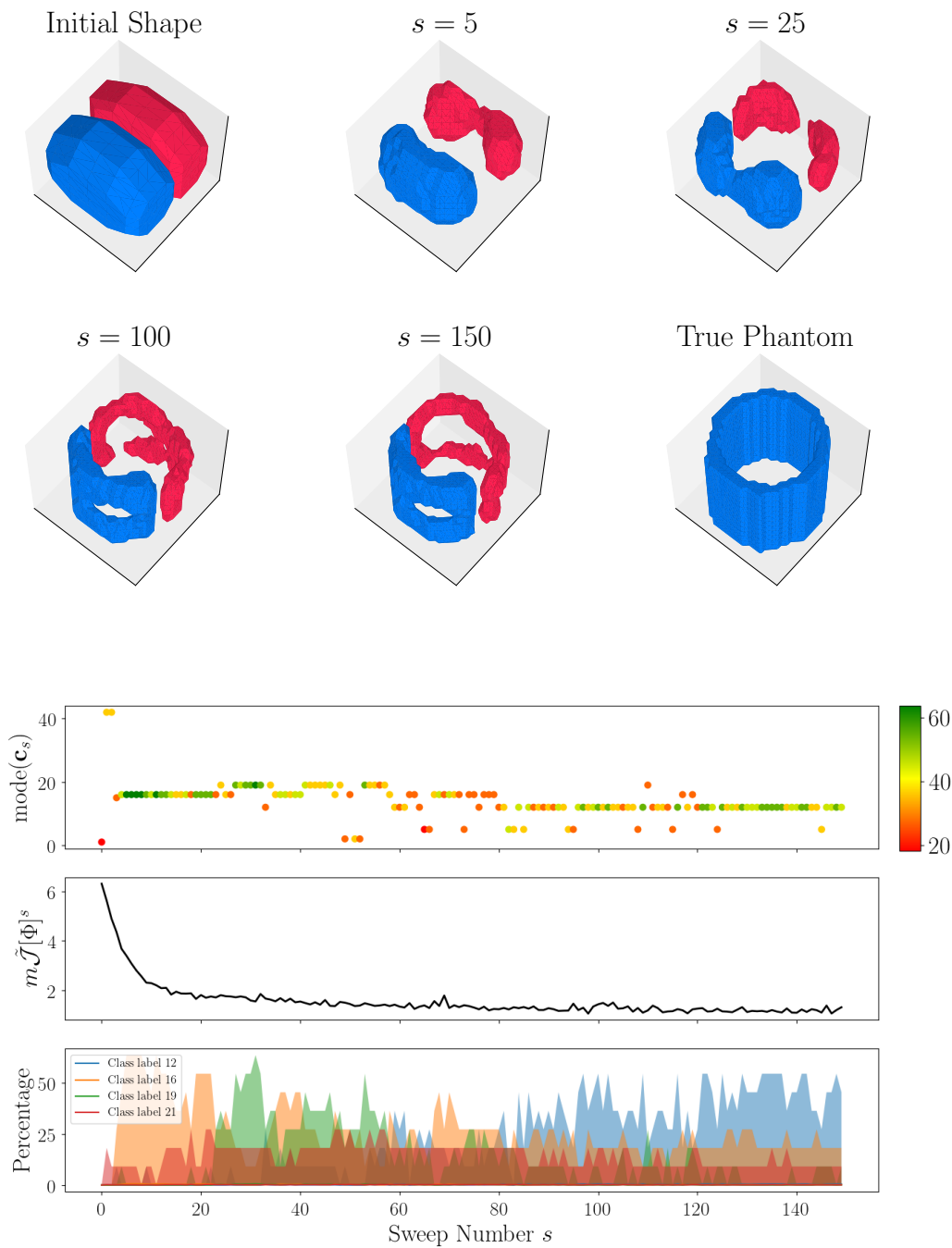
Figure A.9: Top: Surfaces plots of 3D shape evolution using LK-Color level set reconstruction. Shown are the initial shape, snapshots at sweep numbers s = 5, 25, 100, 150 and a true phantom which resembles a capital 'O'.
