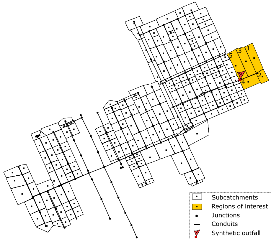
Figure 3. Case study 2 and region of interest highlighted in yellow. The urban drainage system is artificially divided into two sub-systems, with a synthetic outfall (red marker) between them. In this case the region of interest is located in the upstream part of the catchment and has no inflows from upstream. This case study was taken from the work of K. Eckart et al. (2018).
