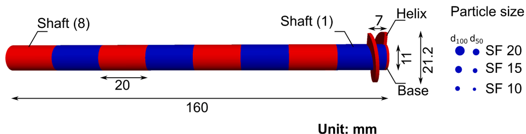
Fig. 2. Pile model and comparison with the particle size at three scaling factors (rotated through 90° in the figure, pile dimensions in mm).
