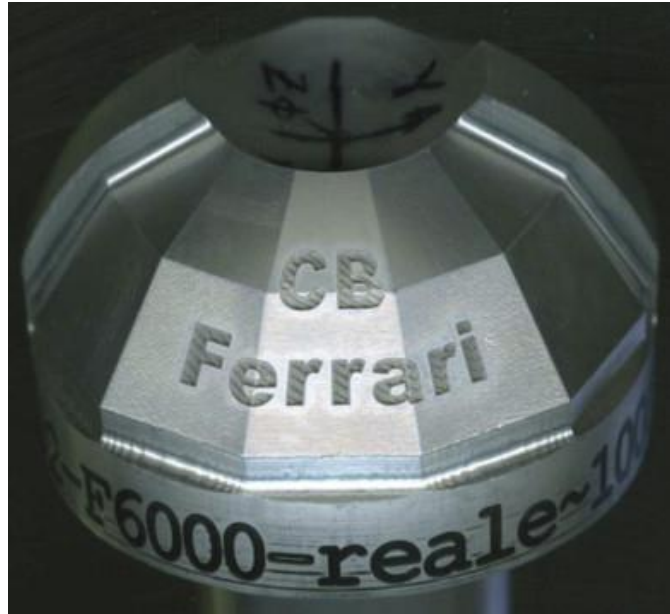
Figure 2.13 Example of a part processed using the CALM software developed by Cuccolini et al. based on the workpiece STL [81]
