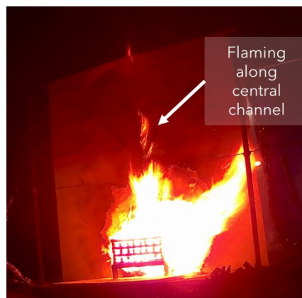
Figure 5.5 - Photo of an experiment with ACP FR (B), Glass Wool (A2) insulation, and a cavity. Flames can be seen ejecting from the small gap between the two panels along the centreline of the facade.
