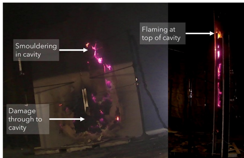
Figure 5.2 - Photos of an experiment with Cement Board (A2) cladding, phenolic foam insulation, and a cavity. Key features from the discussion are labelled.
