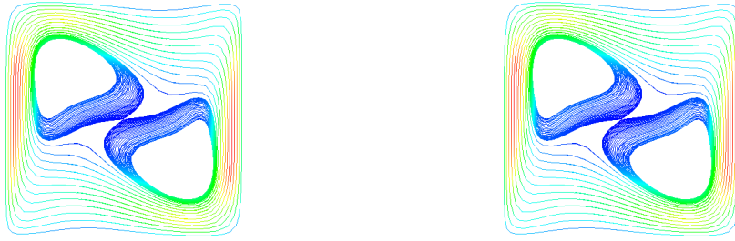
Figure 7.8: Comparison of the velocity streamlines for the full order (left) and reduced order model (right) corresponding to Rayleigh number in the order of 10^5 .
