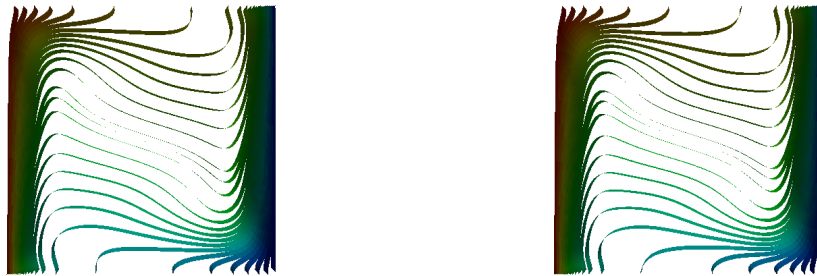
Figure 7.9: Comparison of the temperature isotherms for the full order (left) and reduced order model (right) corresponding to Rayleigh number in the order of 10^5 .
