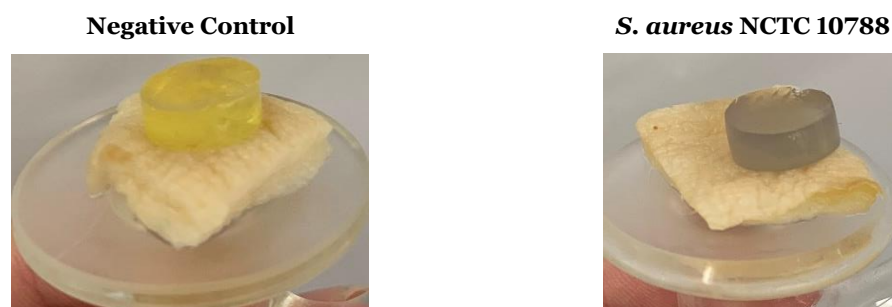
Figure 7.32: 10% w/v PVA hydrogel loaded with 100 \mu\text{M} of TCF-ALP in PBS, pH = 7.4 after 24 h incubation at 32 ^{\circ}\text{C} with porcine skin inoculated with and without S. aureus NCTC 10788.
