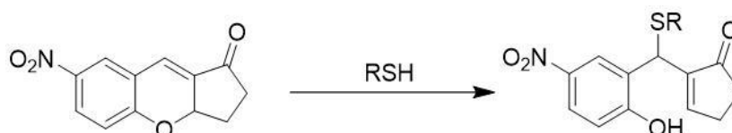
Scheme 5: Michael addition triggered ring-opening reactions to produce 4-nitrophenolate moiety, where -RSH is any thiol containing species. Scheme reproduced from reference Yin et al. 45
