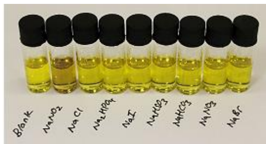
Scheme 3 and Figure 13: Reaction of the azulene chemodosimeter (a) with nitrosonium ion and selectivity of (d) with various anions in solution after 1 minute (left) and 10 minutes (right). Scheme and figure reproduced from reference Lewis et al. 30
