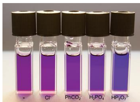
Figure 16: Colour changes of receptors in dimethyl sulfoxide (DMSO) in the absence and presence of anions (3 eq. of TBA salts). Figure reproduced from reference Jurczak et al. 31
