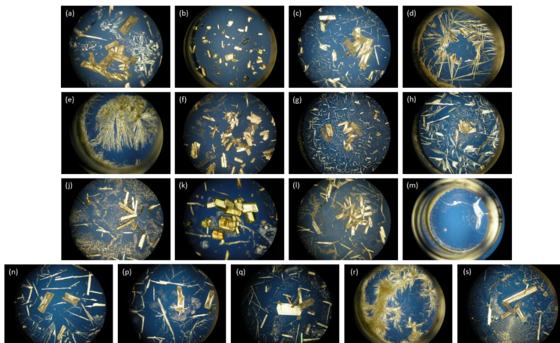
A 3. Evaporative crystallisations at 40 °C with 1% additives (a) benzoic acid, (b) 3-hydroxybenzoic acid, (c) 2,4-dihydroxybenzoic acid, (d) 3,4-dihydroxybenzoic acid, (e) 3,5-dihydroxybenzoic acid, (f) 2,6-dihydroxybenzoic acid, (g) 4-cyanobenzoic acid, (h) 3-cyanobenzoic acid, (j) 2,4-dinitrobenzoic acid, (k) 3,4-dinitrobenzoic acid, (l) 3,5-dinitrobenzoic acid, (m) trimesic acid, (n) isonicotinamide, (p) nicotinamide, (q) pyridoxine, (r) vanillin and (s) L -tartaric acid
