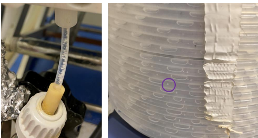
Figure 4.14. Crystallisations in the feed pump outlet (left) and crystals in solution slugs in KRACI tubing (right) for crystallisations of IZN from EtOAc
