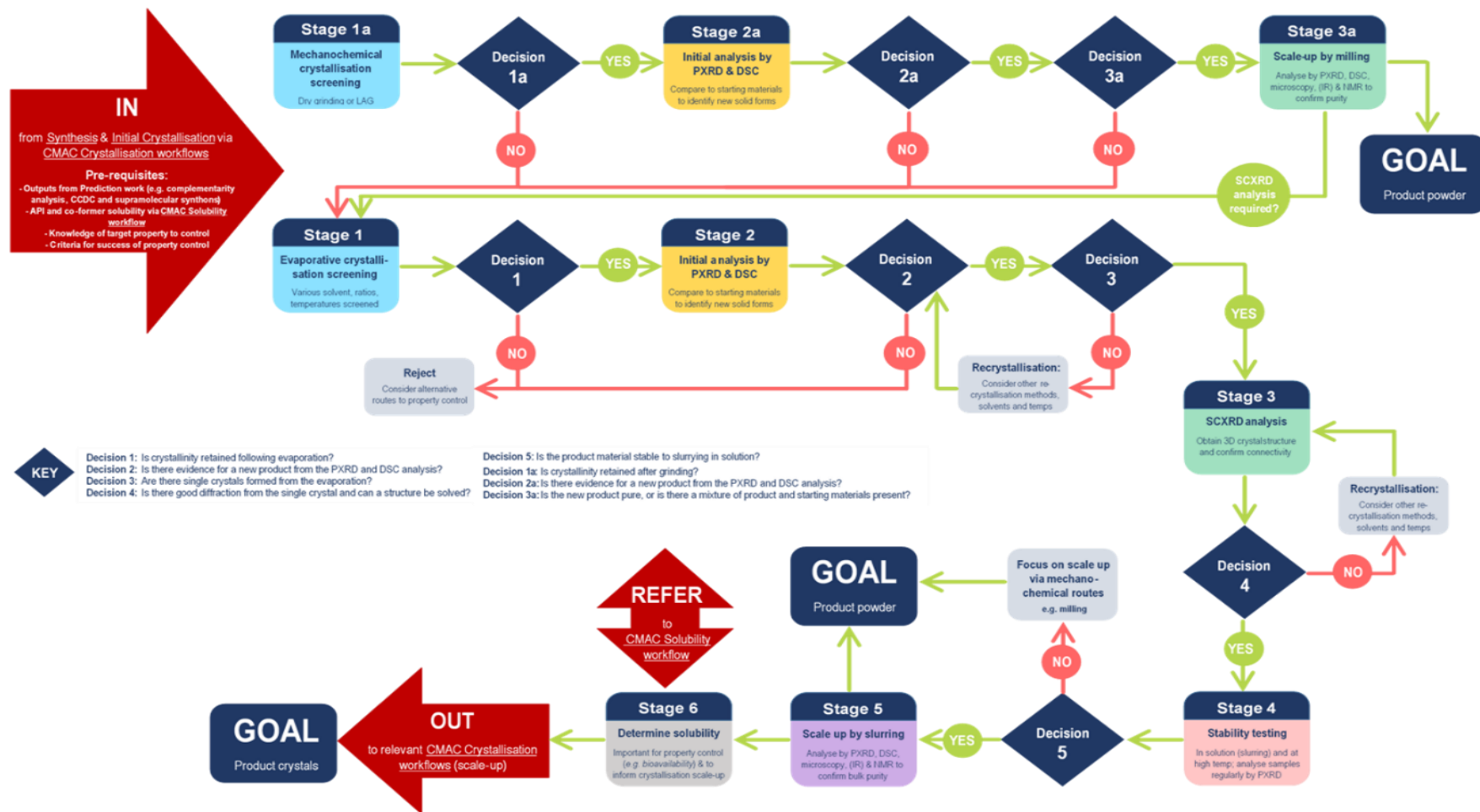
Figure 7.1 CMAC MCM screening workflow driven by the decision points capturing key elements to indicate successes. Decision 1: is crystallinity retained following evaporation?; Decision 2: is there evidence for a new product from the PXRD and DSC analysis?; Decision 3: are there single crystals formed from the evaporation?; Decision 4: is there good diffraction from the single crystal and can a structure be solved?; Decision 5: is the product material stable to slurring in solution?; Decision 1a: is crystallinity retained after grinding?; Decision 2a: is there evidence for a new product from the PXRD and DSC analysis?; Decision 3a: is the new product pure, or is there a mixture of product and starting materials present?
