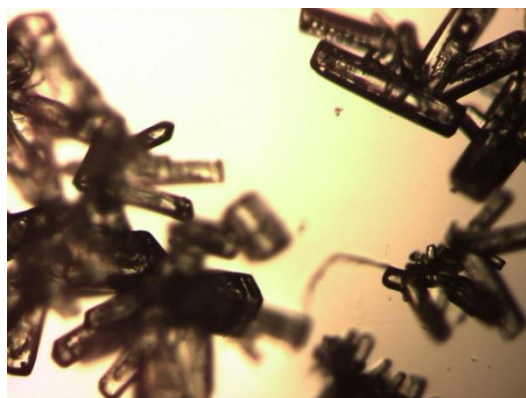
Figure 4.15. Crystals produced from continuous cooling crystallisations from EtOAc in the KRAIC set up
