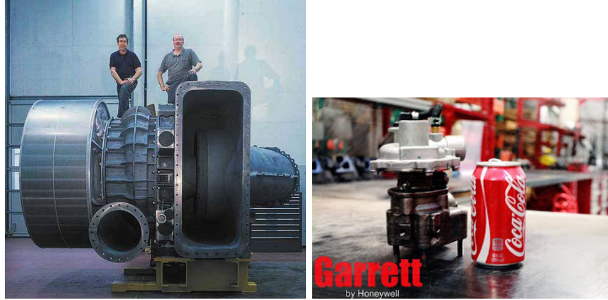
Figure 1-3: Left: Turbocharger for Wärtsilä RT-flex96C engine for a cargo ship [9]. Right: Garrett GT0632SZ turbocharger suited for use with 1L engines [11].
