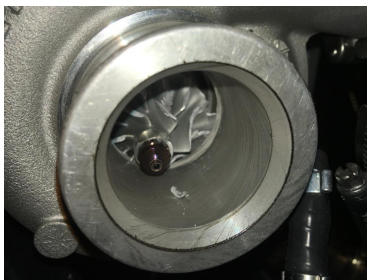
FIGURE 13. TURBOCHARGER FAILURE AS A RESULT OF TESTING AT 135 KRPM.
