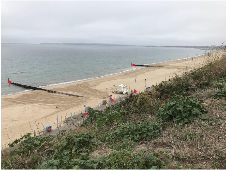
Figure 3.15: An aligned oblique image from Bournemouth showing the 5 GCPs used for rectification, image date: 04/10/18.
