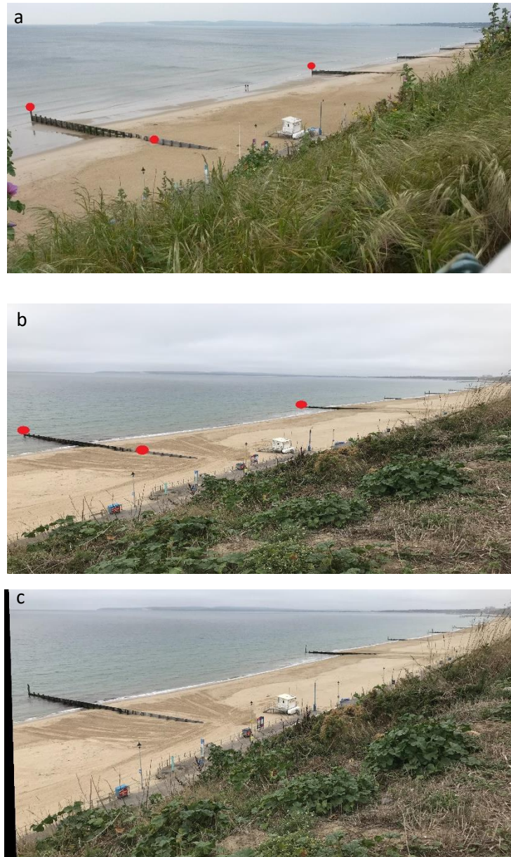
Figure 3.11: a. The alignment points used for Bournemouth images on the baseline image (16/05/18), b. alignment points on an example image (04/10/18) and c. an example aligned oblique image, image date: 04/10/18.
