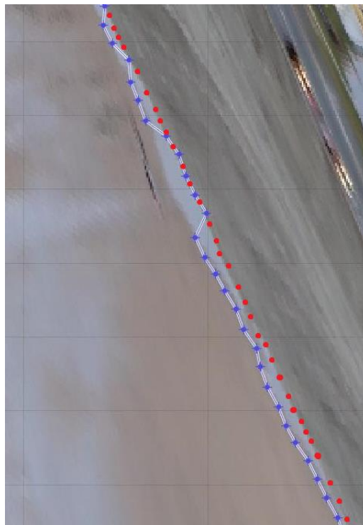
Figure 4.3: An example rectified image showing how the edge detection method (blue line) located the edge of pooled water at the base of the cobble ridge. Red dots show toe of cobble ridge (manually selected). Data from Newgale Cobble toe selections.
