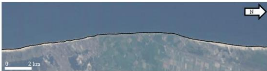
Figure 2.10: a NDWI shoreline detection from Hagenaars et al. (2017) using LANDSAT imagery. The detection works by selecting the location of biggest contrast between land and sea locations.
