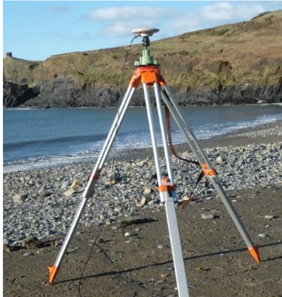
Figure 2.7: An example base station set up at Abereddy using the GPS equipment used in this thesis.
