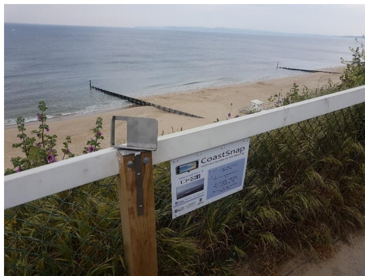
Figure 2.16: CoastSnap Bournemouth camera cradle and sign. The station is situated on top of a cliff looking down onto the beach face.
