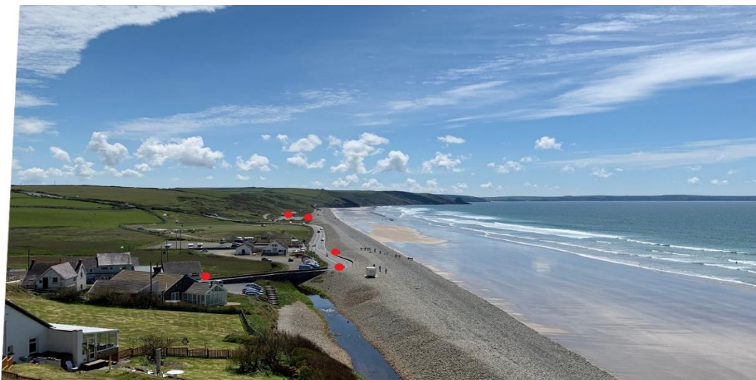
Figure 3.13: An aligned oblique image from Newgale showing the 5 GCPs used for rectification, image date: 23/05/19.
