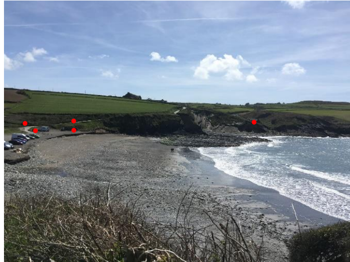
Figure 3.17: The baseline image used for rectification showing the 5 GCPs used for rectification, image date: 6/05/16.
