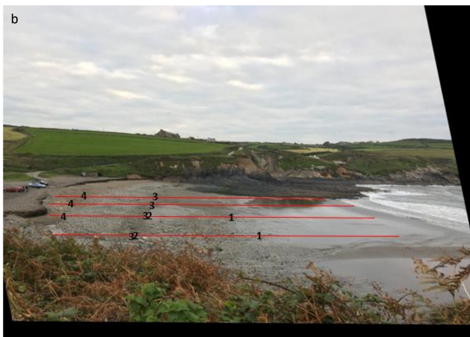
Figure 3.30: a. An example aligned oblique image from Aberreiddy showing three distinct areas of the beach face. Orange section shows location of sparse cobbles, green section shows location of no cobbles (i.e. sand) and blue section shows location of dense cobbles (i.e. cobble ridge). b. The same aligned oblique image from Aberreiddy showing the u , v points obtained. The numbers relate to the points identified in Section 3.4.3.1. Note that some transects in this example do not have sparse cobbles and that in some cases the end of the sparse cobble point and the start of the dense cobble point are in the same location, e.g. transects closest to camera. Image date: 7/10/16.
