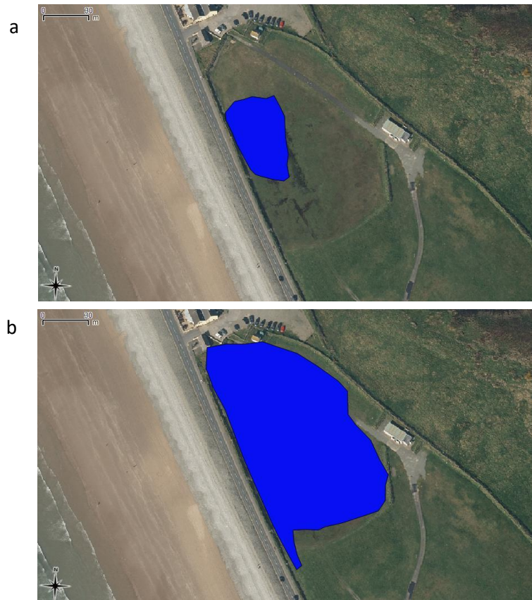
Figure 4.12: Flood extent layers for different images at Newgale with Digimap imagery (2020) used as backdrop. a. 24/03/17 and b.03/01/18.
