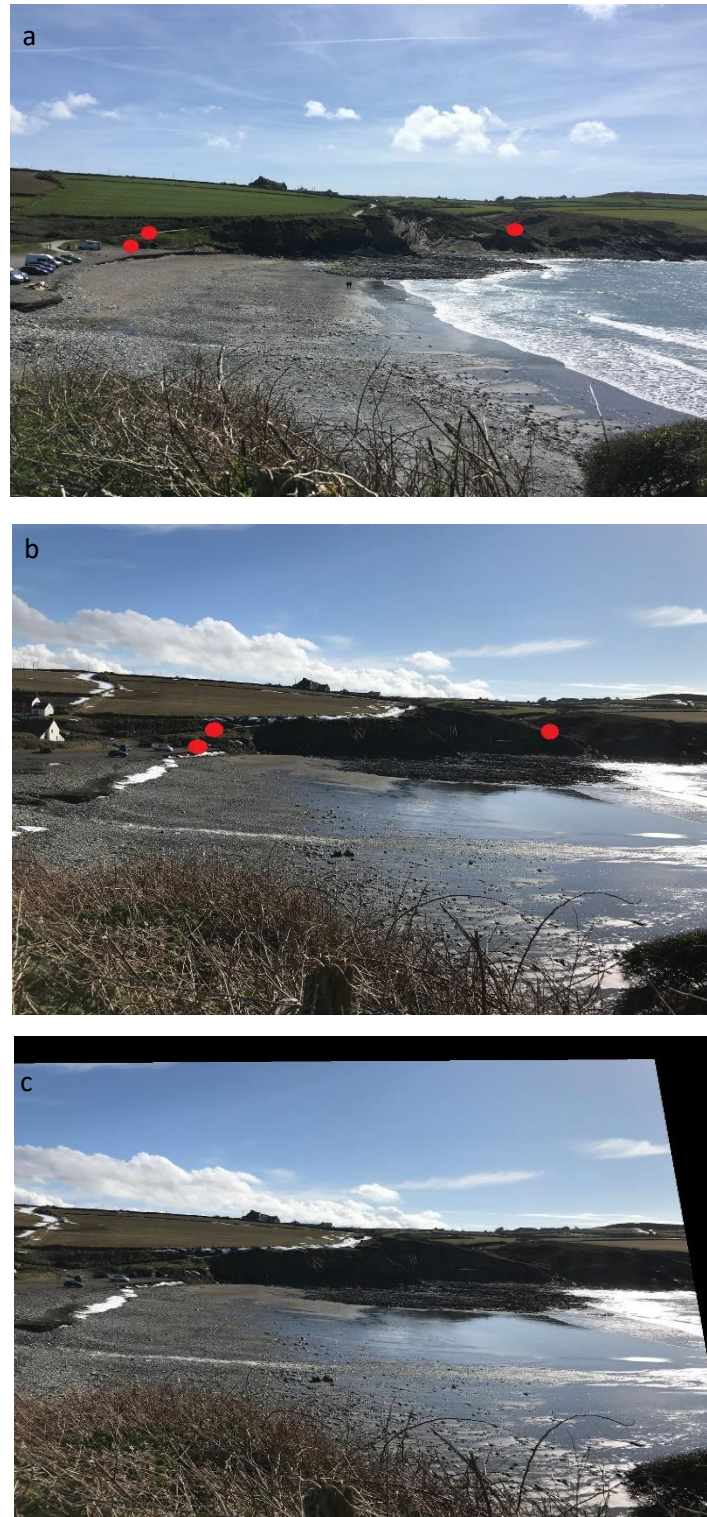
Figure 3.12: a. The alignment points used for Aberreiddy images on the baseline image (6/05/16), b. alignment points on an example image (4/03/18) and c. an example aligned oblique image, image date: 4/03/18.
