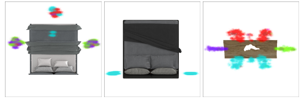
Figure 5: Example layout patterns between dominant objects and subordinate objects: Double Bed & Rug (Left), Double Bed & Nightstand (Middle), Dining Table & Chair (Right). Colors denote orientations of sub-object following HSV color space where pure cyan is 0 degree.
