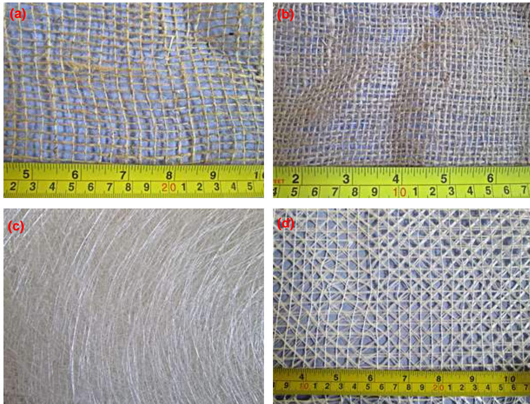
Figure 4: Type of reinforcements. Traditional hessian fabric - (a) Loose weave hessian and (b) Plain weave hessian; Modern glass fabric - (c) Continuous fibreglass mat (CFM) and (d) Quadaxial glass fabric
