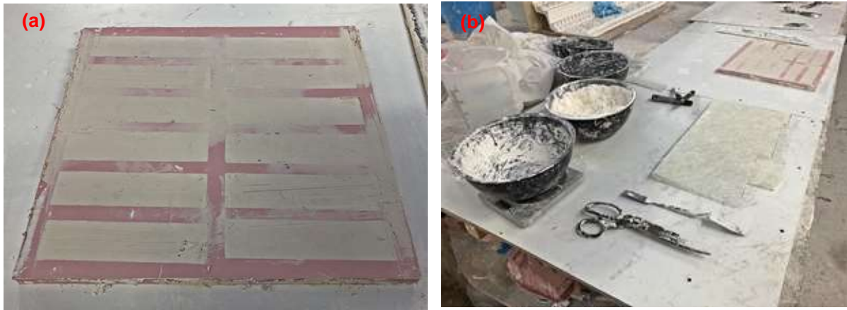
Figure 5 : Manufacture of fibrous plaster specimens showing (a) plaster in a silicone mould and (b) plaster and glass reinforcement materials used in the process
