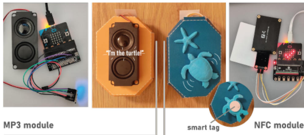
Figure 3.16: Modules of Sound and identification with NFC. The prototype is made in blue and orange cardboard, and inside, it carries the corresponding hardware components. The smart tag is a sticker on the animal's bottom part, identified by proximity when placed above the NFC reader.
