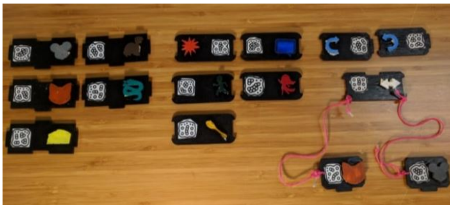
Figure 2.5: Blocks used in the initial StoryBlocks prototype include characters (mouse, turtle, cat, snake, cheese), actions (explode, talk, run, dance, eat) and control structures (repeat, branch).
