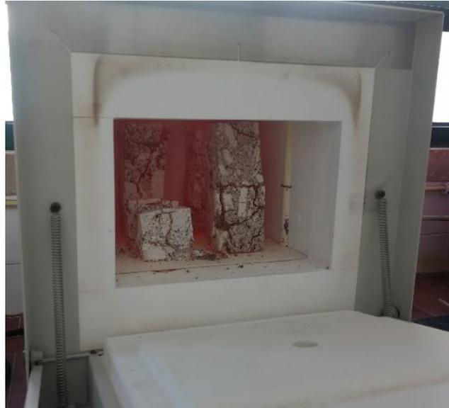
Figura 4.2.1: Mufla *EHRET MUFFLE FURNACE* (modelo MO L 3; 5; 9;11/ S27) da *Nabertherm*.
