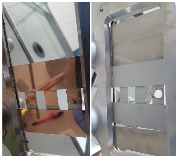
Figure 4.7: Before (left picture) and after (right picture) evaporation of natural Sn on Cu backing.
