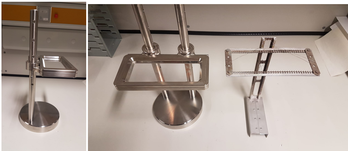
Figure 4.1: Comparison of the new and old evaporation supports used to produce the target. Left picture: side view of the new support. Right picture: front view of the new (left) and old (right) supports.
