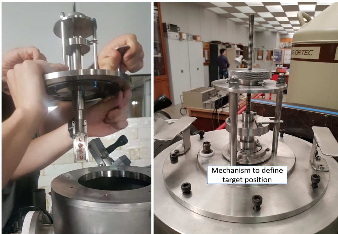
Figure 4.13: left - Picture of the target holder being removed from inside the chamber. Right - Target holder placed inside the chamber.
