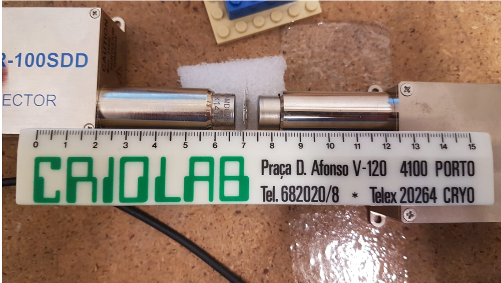
Figure 4.22: Decay acquisition setup at FCUL with two detectors: the XR-100SDD (left side) and the SXD15M-150-500 (right side).
