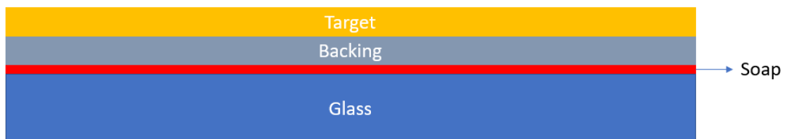
Figure 4.5: Figure representing the layer composition before fishing the targets
