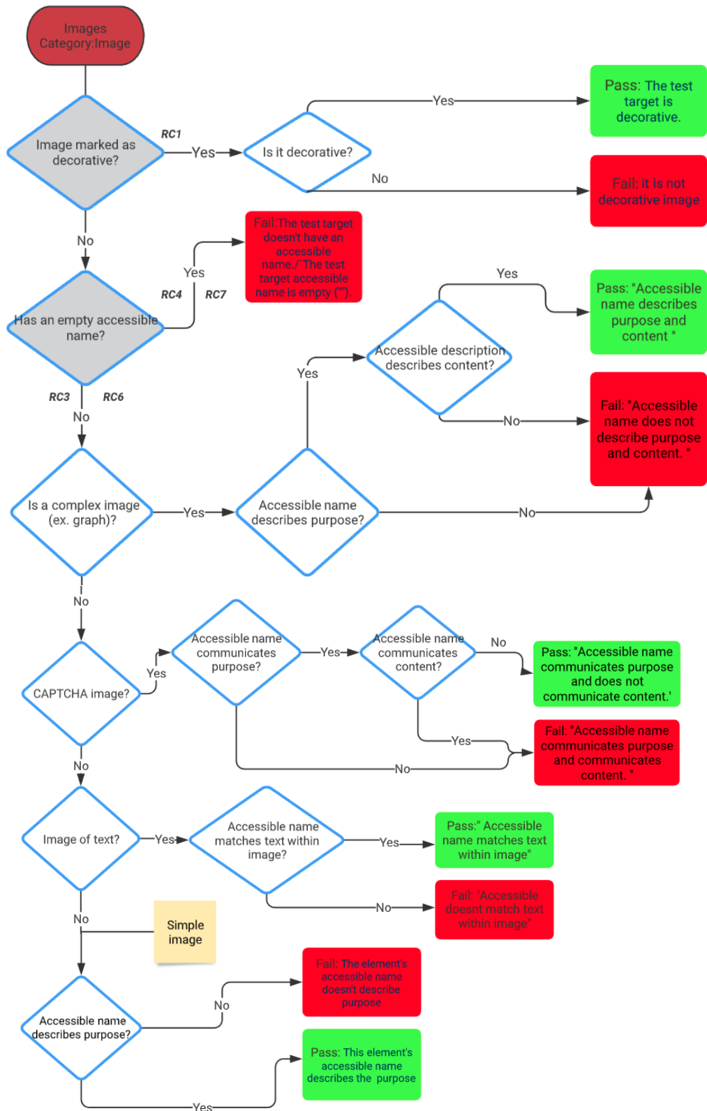
Figure 4.3: Diagram flow of Rule 17. This rule checks that each image either has a non-empty accessible name or is marked up as decorative.
