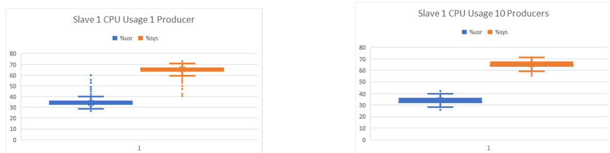
Figure 6.8: Slave 1 - CPU level - 1 Producer vs 10 Producers
