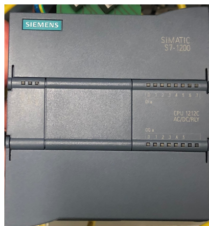
Figure 2.4: SIMATIC S7-1200 PLC
