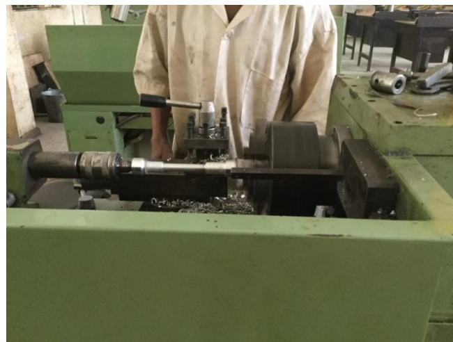
Figure 6: Machining the tensile shape with the lathe machine
