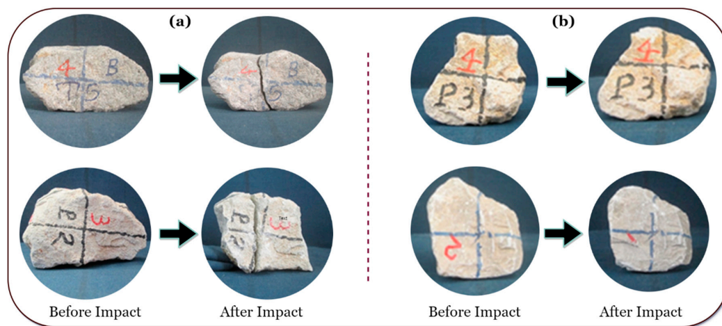
Figure 9. Comparison of ballast degradation patterns: (a) fragmentation; (b) abrasion [18].
