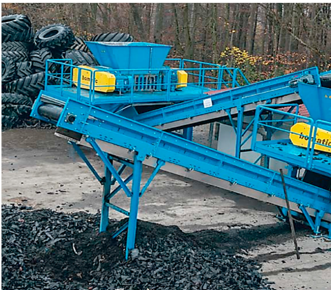
Fig. 3. Rubber tire shredder (source: Weber and Kroll, 2019).
