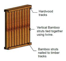
Figure 4.25: Walling Components made with Bamboo Sticks
