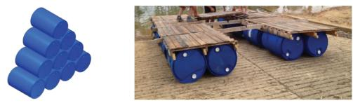
Plate 4.2: Plastic Barrel used to achieve Buoyancy Source: [20].
