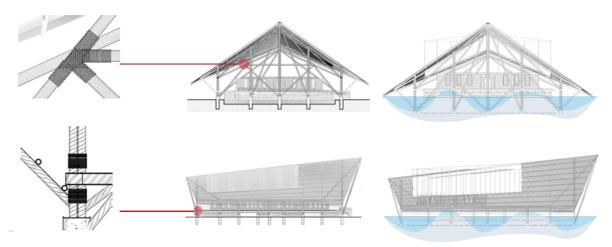
Figure 4.9: Platform Design Schematic Diagram
