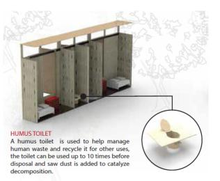
Figure 4.31: Humus Toilet Positioned in a Structure
