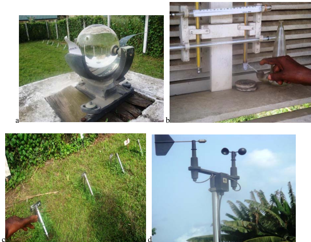
Figure 1: Equipment at NIMET a, Campbell-Stokes sunshine recorder b, Stephenson screen thermometers c, soil thermometers d, anemometer
