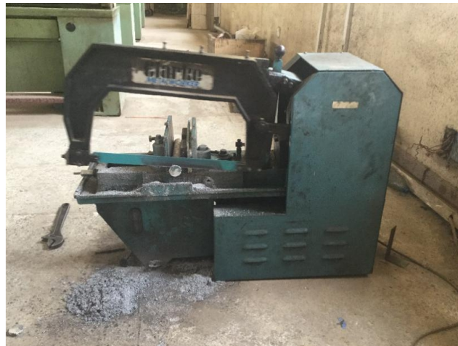
Figure 5: Circular shapes cut using a power hacksaw
