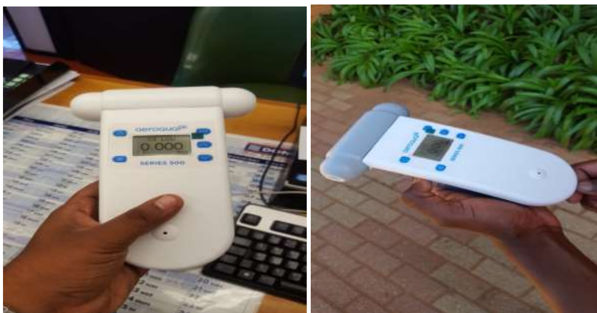
Figure 3.4: Indoor and outdoor pollutant sampling using the Aeroqual portable handheld meter.
