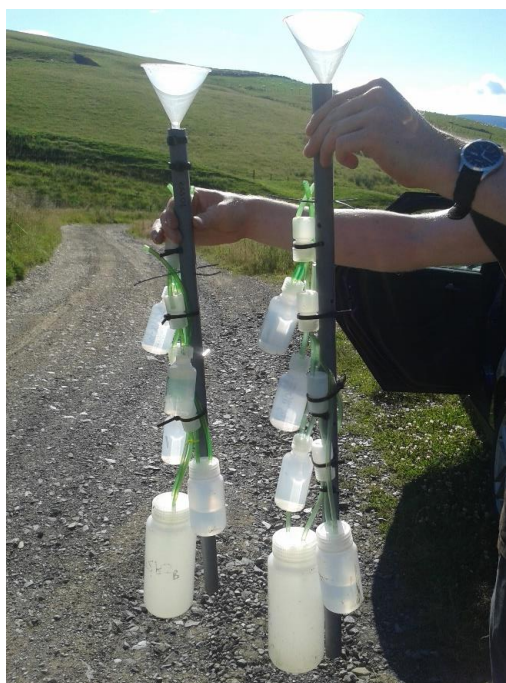
Figure 4.2: The internal structure of the two sequential rainfall samplers following the July 2016 event.
