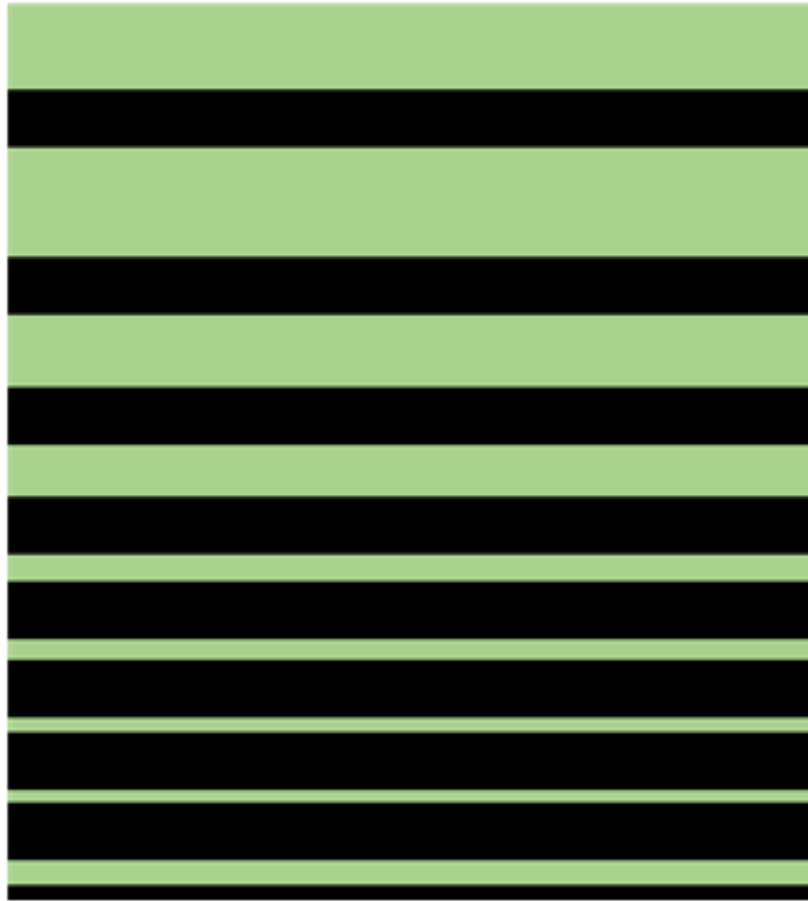
Figure 8.2 The image applied to the sample by the digital mirror device comprising of a series of dark bars of width \sim 50 \mu\text{m} spaced by a range of illuminated bars of widths ranging from 25 to 225 \mu\text{m} , where the entire image is 1.10 \times 0.93 \text{ mm}^2 . The patterns shown correspond to the field of view.
