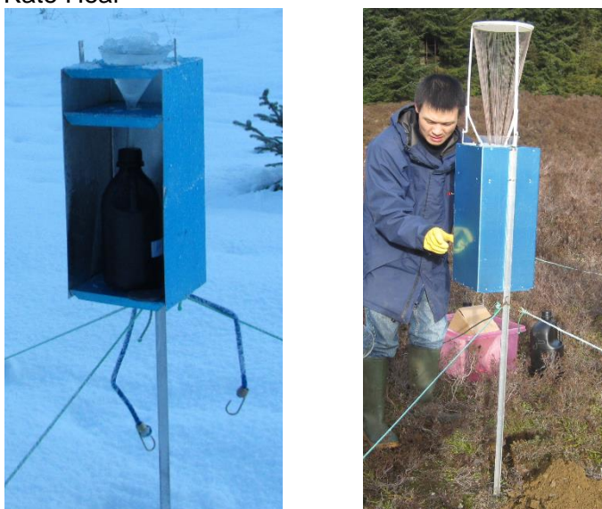
Figure 2-4. Rainfall (left) and harp-wire cloud/fog collector at Griffin upper site. Photo: Kate Heal
