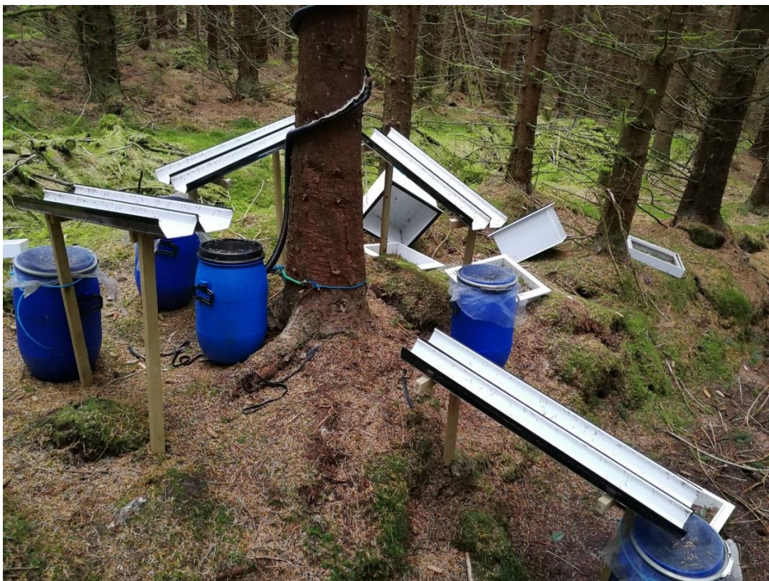
Figure 4-2. TF collectors and SF collector under T2, April 2017
