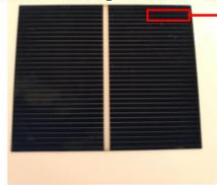
Fig. 6. (a) Cracked solar cell tested under STC, (b) PV Class AAA Flasher setup
