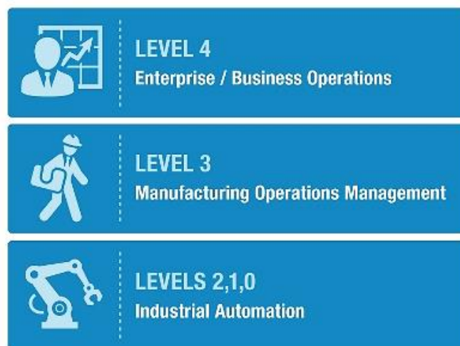
Figure 1 ANSI/ISA-95 functional hierarchy model (ISO British Standards Institution, 2018)
