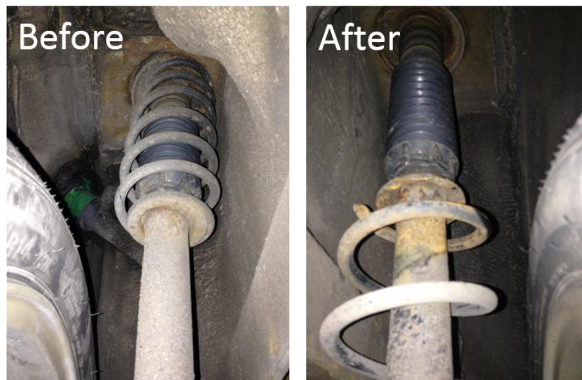
Figure 1. 1. Suspension failure due to extensive corrosion of the author's car.
