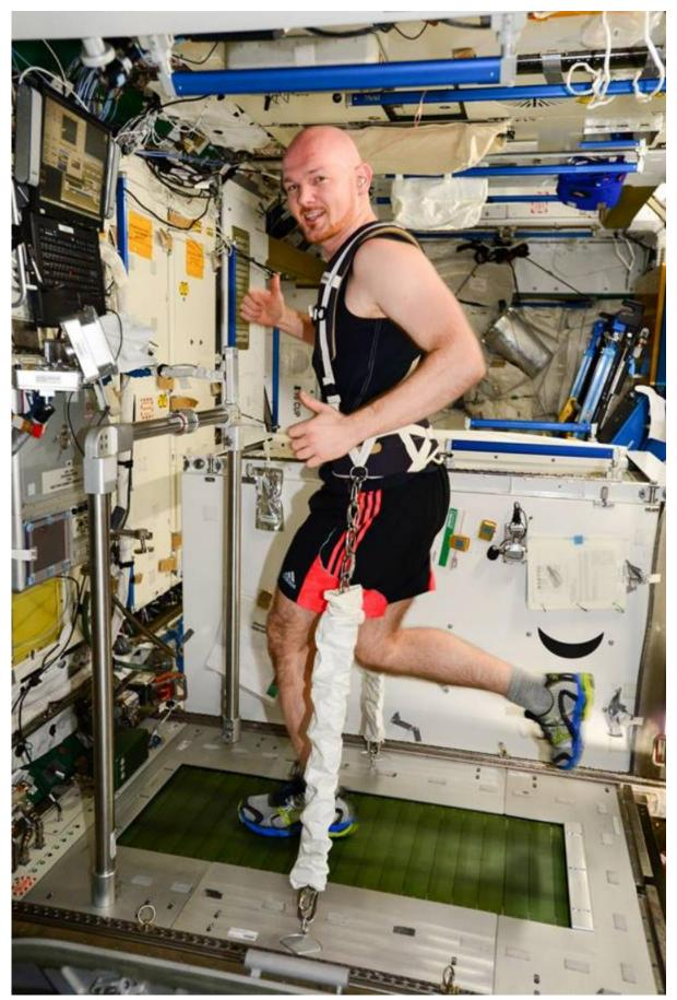
Figure 1 T2 running system with harness, bungee assembly and carabiner clips (with friendly permission by A. Gerst / ESA).
