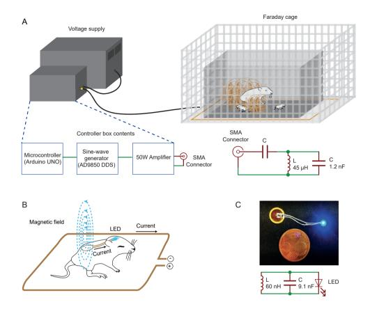
Figure 1, Resonant-induced current activates a wireless implanted LED
