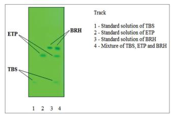
Fig. 1: Thin-layer chromatography plate of terbutaline sulfate, etophylline, and bromhexine hydrochloride
