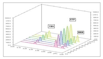
Fig. 3: Overlay linearity chromatogram of terbutaline sulfate, etophylline, and bromhexine hydrochloride 60-210 ng/band, 2400-8400 ng/band, and 96-336 ng/band, respectively
