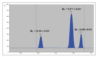
Fig. 2: Typical chromatogram of terbutaline sulfate  $R_{\rm j}{=}0.24{\pm}0.02$ , ETP  $R_{\rm j}{=}0.57{\pm}0.02$ , and BRH  $R_{\rm j}{=}0.68{\pm}0.02$
