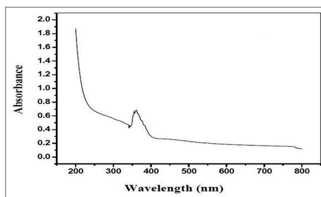
Fig. 1: UV-visible spectrum of synthesized zinc oxide nanoparticles
