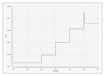
Fig. 9: Voltage transient characteristics of Model 1 low dropout regulator
