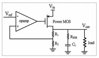
Fig. 1: Basic low dropout schematic
