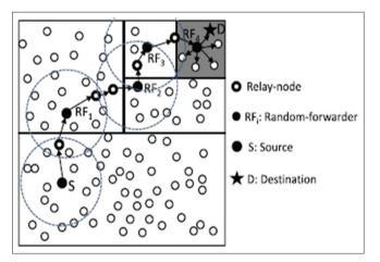
Fig. 6: Routing among zones in anonymous location-based efficient routing protocol
