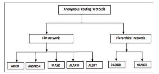
Fig.1: Classification of anonymous routing protocols in mobile ad hoc network
