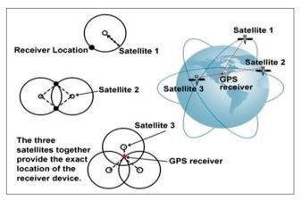
Fig. 1: Working of global position system
