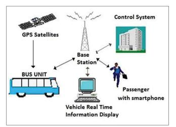
Fig. 2: Architecture of proposed system
