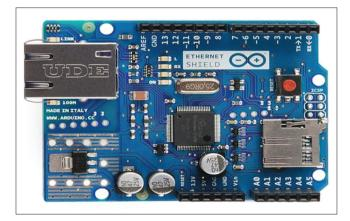
Fig. 4: Ethernet shield
