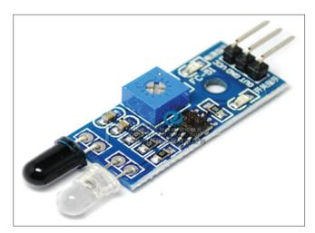
Fig. 5: Infrared sensor
