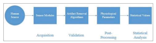
Fig. 5: Processing steps of biosignals according to the proposed layer model. Specific sensors are applied to a physiological system and their response to changes within this system is recorded and digitalized, yielding digital biosignals (in the acquisition layer). After cleaning signals from artifacts and synchronizing (validation layer), the validated signals can be used for the calculation of physiological parameters
