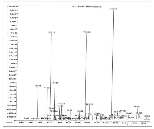
Fig. 1: Gas chromatography-mass spectrometry analysis on ethyl acetate extract of Garcinia mangostana leaves
