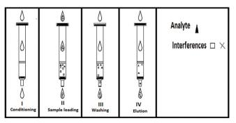
Fig. 1: Steps in solid phase extraction
