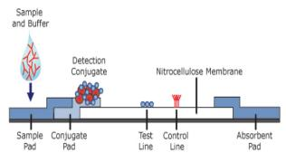
Fig. 2: Diagram of the lateral flow immunoassay (Reproduced from: web)
