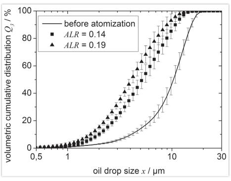
Figure 5: Oil drop size distribution of an oil in water emulsion before (continuous line) and after atomization (discrete data points) by an effervescent atomizer at two different ALR [7].
