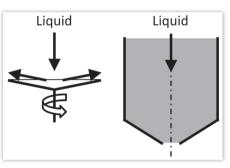
Figure 1: Schematic drawing of a rotary atomizer (left) and a pressure nozzle (right).
