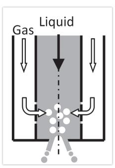
Figure 3: Schematic drawing of an effervescent atomizer (according to [5])
