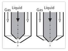
Figure 2: Schematic drawing of a pneumatic nozzle with internal (left) and external (right) mixing.
