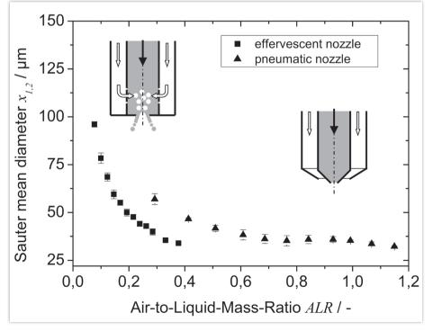
Figure 4: Impact of ALR on the Sauter mean diameter of the spray droplets atomized by an external mixing pneumatic nozzle and an effervescent atomizer at constant liquid flow (liquid viscosity: 25.5 mPas) [6] DryConsult International ApS, Charlottenlund, 2002
